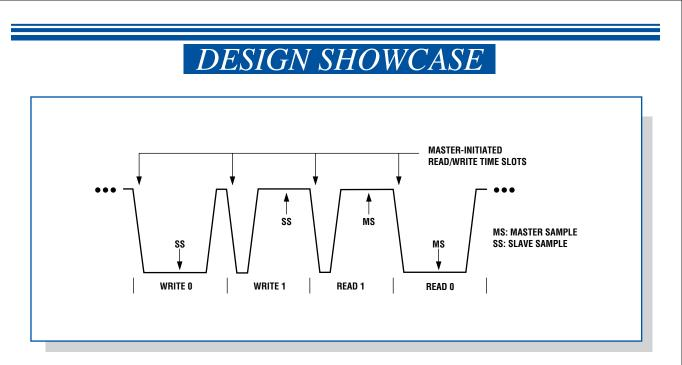
Figure 2. This waveform example shows master-initiated write/read of data bits with slave and master sampling points.
