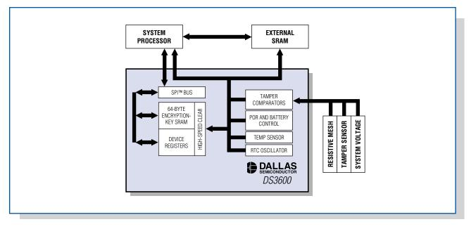
Figure 1. The tamper-resistant DS3600 controller features extremely high-impedance comparators to provide continuous low-power system monitoring and meet the highest level Common Criteria requirements.
