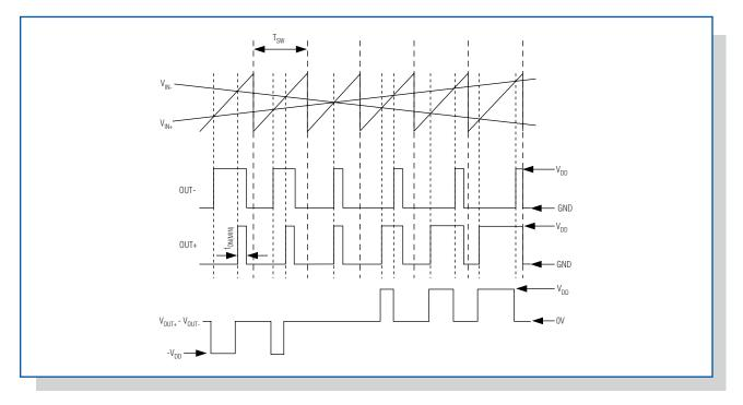
Figure 8. The input and output waveforms are shown for the MAX9700's filterless modulator topography.
