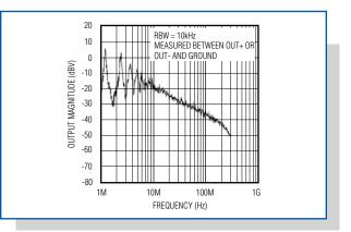
Figure 9b. Spread-spectrum modulation redistributes the spectral energy of the MAX9700 over a wider bandwidth.
