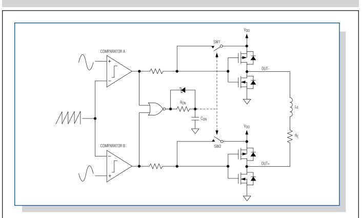
Figure 7. This simplified functional diagram shows the MAX9700's filterless Class D modulator topography.
