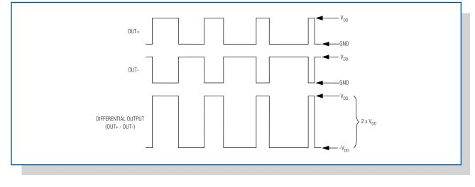
Figure 6. Traditional full-bridge Class D output waveforms complement each other, thus creating a differential PWM signal across the load.
