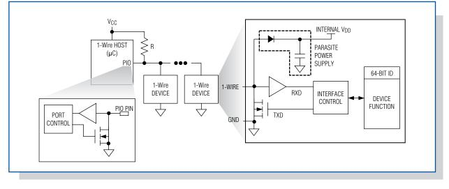
Figure 1. In a 1-Wire master/slave configuration, all devices share a common data line.
