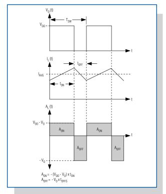
Figure 3. Filter inductor current and voltage waveforms are shown for a basic half-bridge Class D amplifier.
