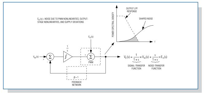
Figure 4. A control loop with 1st-order noise shaping for a Class D amplifier pushes most noise out of band.
