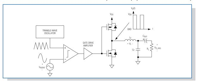
Figure 1. This simplified functional block diagram illustrates a basic half-bridge Class D amplifier.
