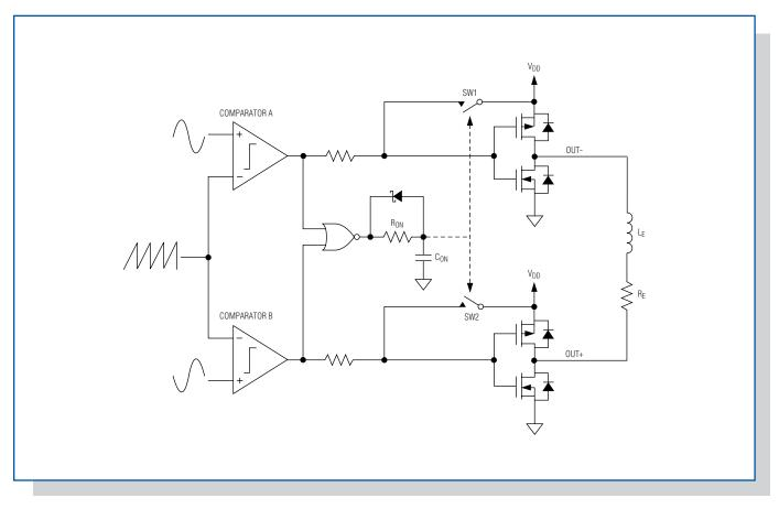
This simplified functional diagram shows the MAX9700's filterless Class D modulator topography. (See page 8.)
