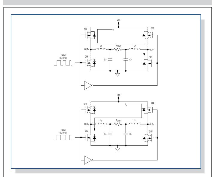
Figure 5. A traditional full-bridge Class D output stage uses two half-bridge stages to drive the load differentially.
