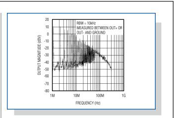
Figure 9a. The wideband output spectrum is shown for the MAX9700 using a fixed switching frequency.
